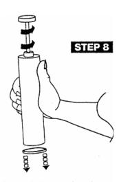
Remove bottom cap from the cartridge and unscrew the rod from the wheel in a counter-clock wise direction. Remove the rod from the cartridge and discard.
