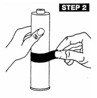
Remove tape band from the cartridge kit and discard.
