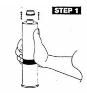
Remove Red Snap Lock Plug from top of cartridge.
