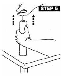
Pull rod straight up towards open end of cartridge. This will separate the foil from the mixing wheel.
