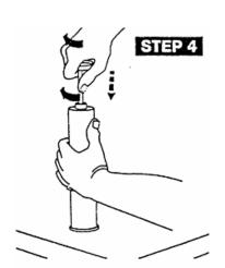
Insert plunger rod through opening and fasten rod to wheel by turning clockwise approximately three (3) turns.
