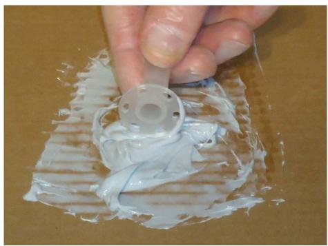
Roll the base of the port in mixed #602 along the edge – make sure not to plug hole in center of base.
