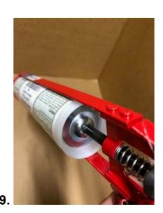
Make sure the wall crack is at least 1/32" wide before injecting. Space injection ports 6" apart or closer.
