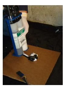
Remove strap and plug of each port. Put the plugs in your shirt pocket for quick access.
